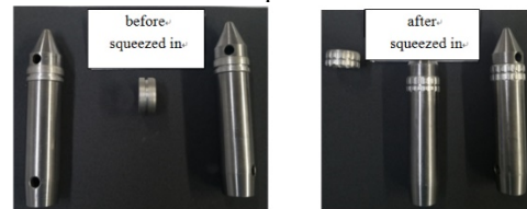
(2) Comparison of before and after extrusion of duralumin 2A-12 material belt
