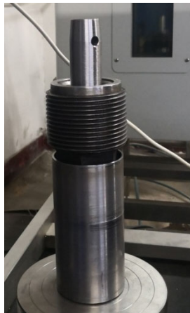
Figure. 4 The actual picture of the assembly of the extrusion test device
