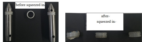
(3) Comparison of nylon Nylon1010 material belt before and after extrusion
