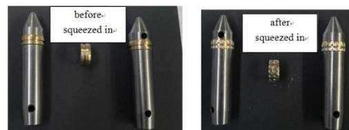
(1) Comparison before and after the brass H96 material belt is squeezed in
