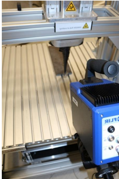
Fig. 3. Infrared camera recording process of sample excitation.
