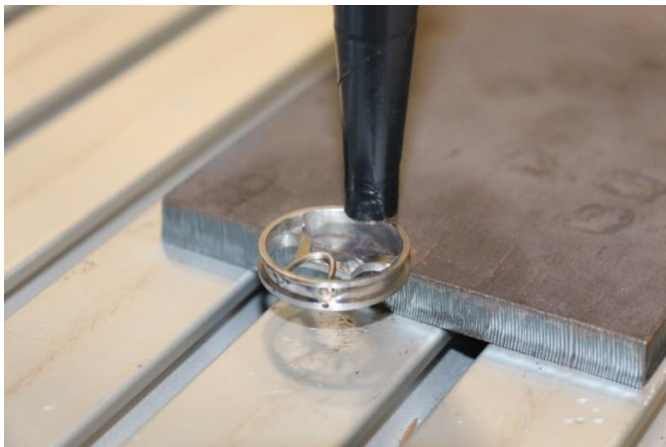
Fig. 2. The sample under ultrasound exciter.
