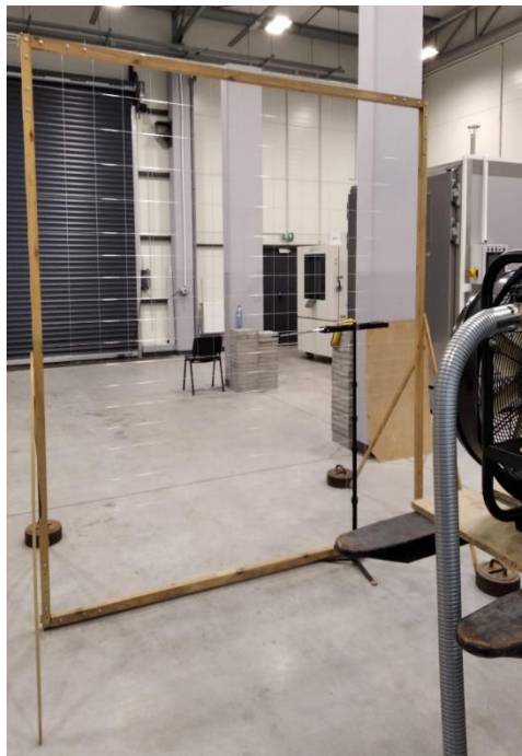
Fig. 2. Test stand (measurement plane) for assessing the characteristics of velocity profile of the air stream generated by the mobile overpressure fan.
