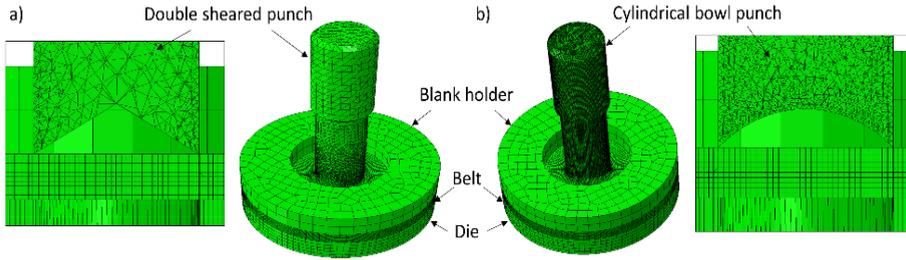
**Fig. 3.** FEM model construction.
