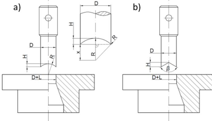
**Fig. 1.** Axially non-symmetrical punches cooperating with a die a) double sheared punch, b) cylindrical bowl punch: D – punch diameter, H – shearing/bowl height, L – punch-die clearance,  $\beta$  – tip angle, R – bowl radius.
