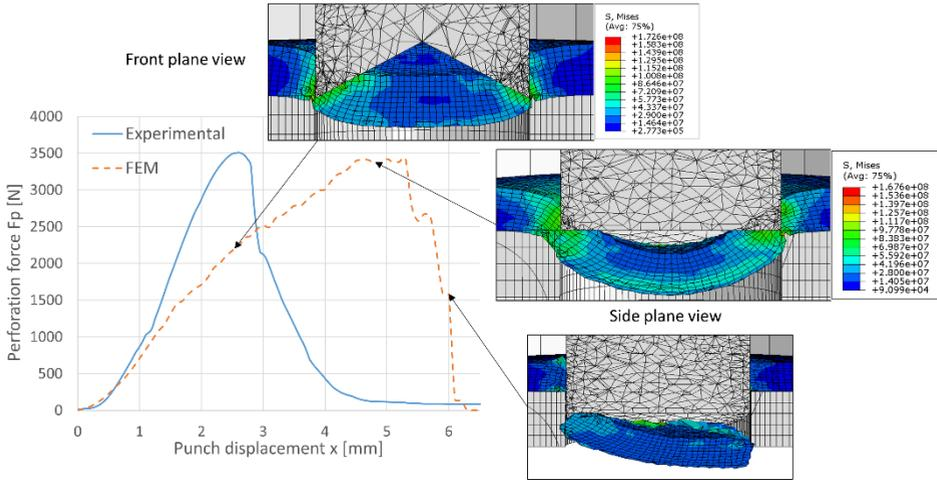
**Fig. 4.** Comparison of FEM and experimental results for TFL10S belt perforation with a double shear punch with a tip angle  $\beta = 120^\circ$  along with sample stress distribution obtained from FEM analysis.
