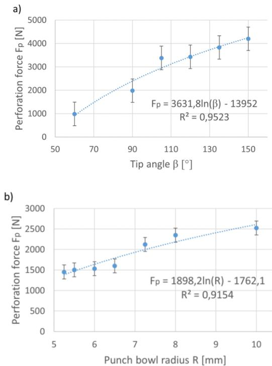
**Fig. 6.** The influence of the tip angle  $\beta$  (a) and bowl radius  $R$  (b) on the perforation force  $F_P$  for axially non-symmetrical piercing punches.
