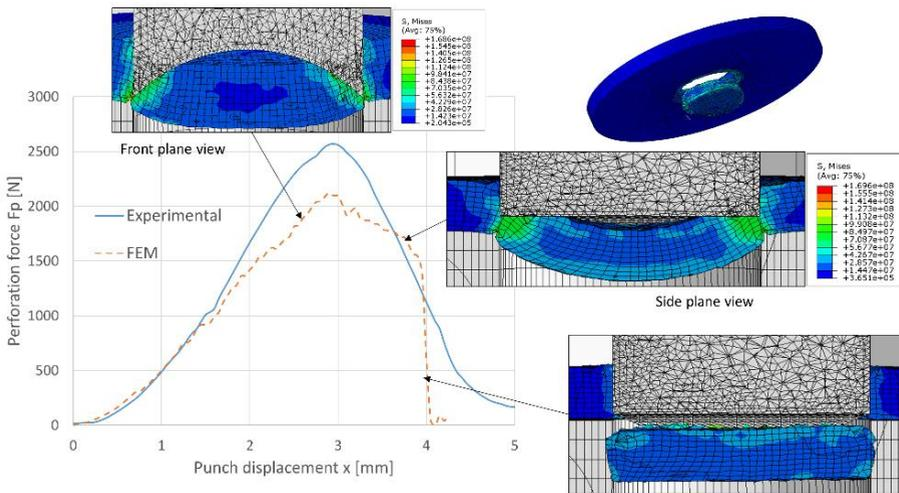
**Fig. 5.** Comparison of FEM and experimental results for TFL10S belt perforation with a cylindrical bowl punch with bowl radius  $R = 7.25$  mm along with sample stress distribution obtained from the FEM analysis.
