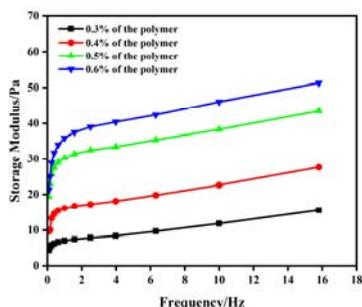
**Fig. 2.** Elastic modulus test curves for different polymer concentration systems.
