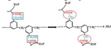
**Fig. 1.** Schematic diagram of gel reaction mechanism.
