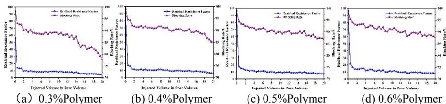
**Fig. 3.** Scour resistance curves of gels with different polymer concentrations.
