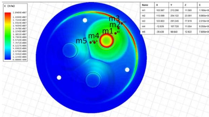
**Fig. 9** Field strength distribution on concave surface of pot insulator
