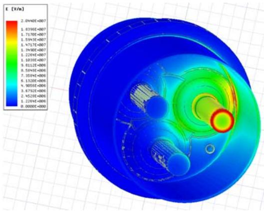
**Fig. 6** Phase A is pressurized, phase B / C is grounded, the electric field is distributed as a whole
