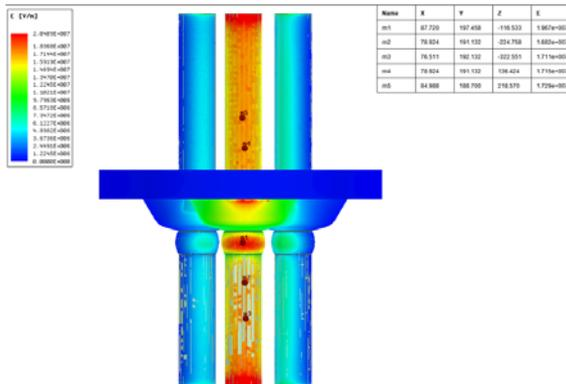
**Fig. 7** Field strength distribution on conductor surface
