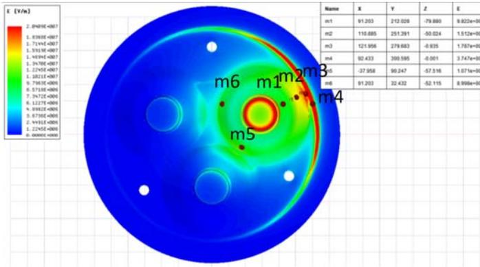
**Fig. 8** Field strength distribution on convex surface of pot insulator
