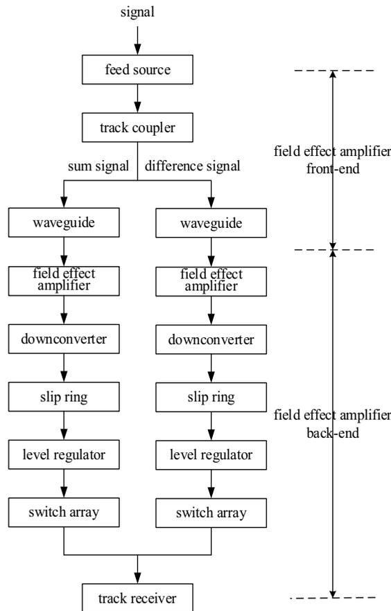
Fig. 1. Signal transmission channel.
