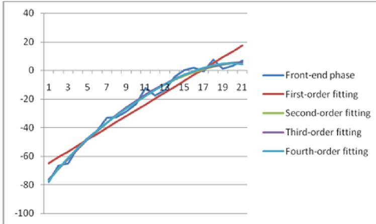
**Fig. 2.** Phase fitting results of the of the field effect amplifier front-end.
