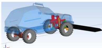
Fig. 2. An illustration of a MBS model of the investigated off-road vehicle in the Simpack software.
