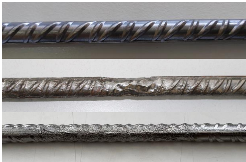
Fig. 5. Non corroded steel bar (up), corrosion damage on short exposed length (middle) and corrosion damage on long exposed length (bottom)
