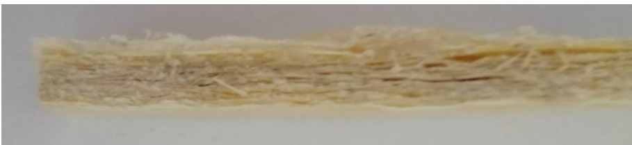
Fig. 7. Defects in samples after cutting them from the plate
