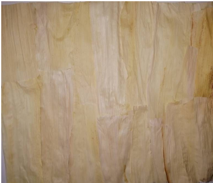
Fig. 1. A sheet from epoxy resin and corn ear leaves
