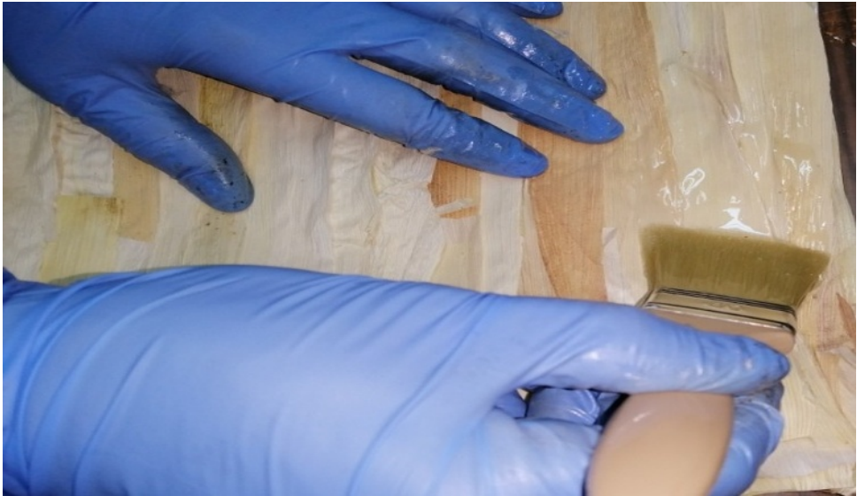
Fig. 2. Applying the epoxy resin on the created sheets (paper+corn ear leaves)
