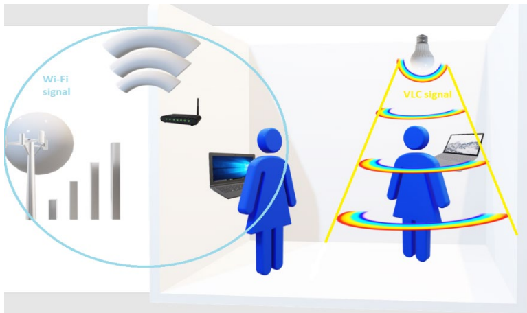
Fig. 2. Wi-Fi signal configuration versus a VLC signal in a LoS scenario
