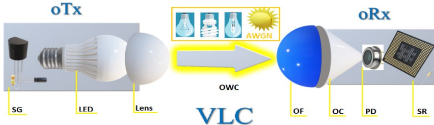
Fig. 1. General configuration of a VLC system with LoS topology
