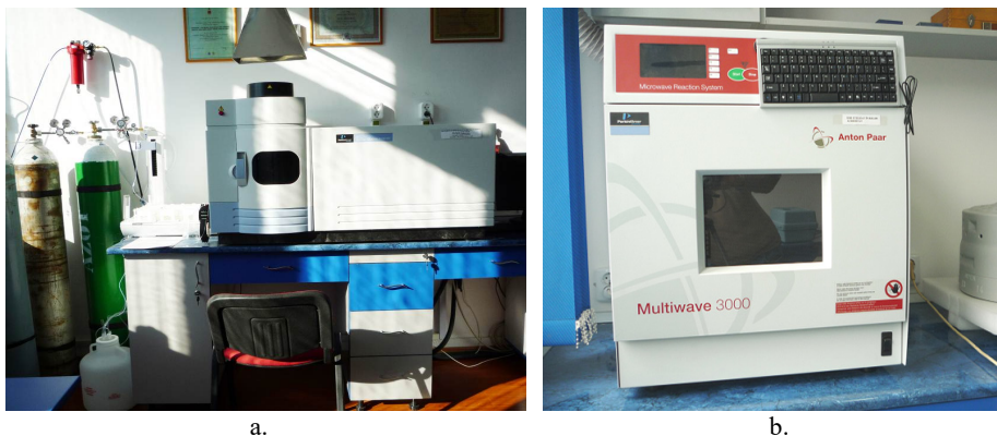
Fig. 3. Inductively coupled plasma optical emission spectrometer ICP-OES Perkin Elmer (a), Microwave oven for solid sample digestion (b).
