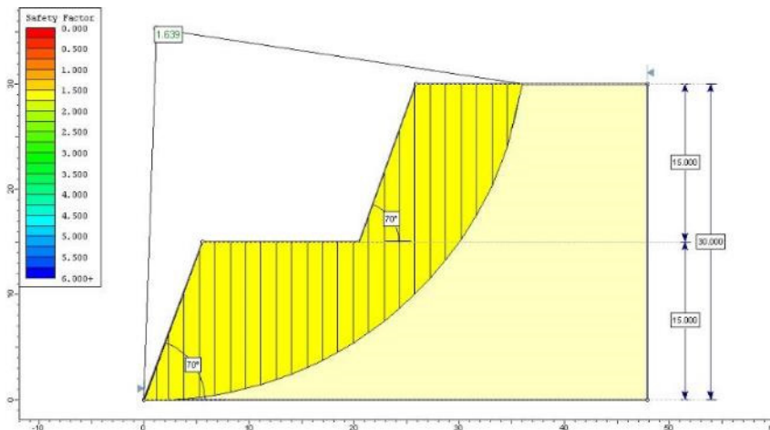
Fig. 9. Safety factor for two-bench system by Janbu' method.
