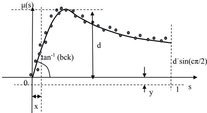
Fig.3. The “Pacejka magic formula” explanation [5] data from experiments. The force for “zero slip” is flowing – describe by one of adjustable parameters.
