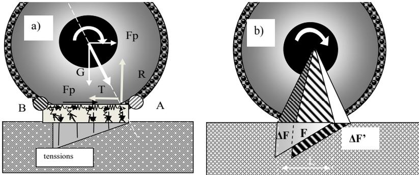
Fig.6. Force layout under rotating wheel [13]
