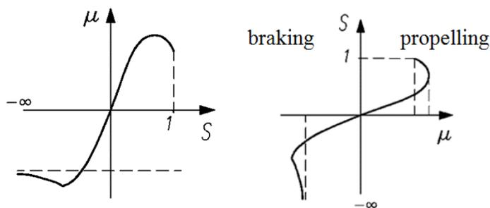
**Fig. 1.** Diagram of the wheel's slip as a function of the propelling force coefficient [5].
