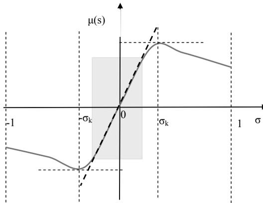
**Fig.4.** Classical relation curves of driving force coefficient ( $\mu$ ) to slip ( $s$ )  $\mu=f(s)$
