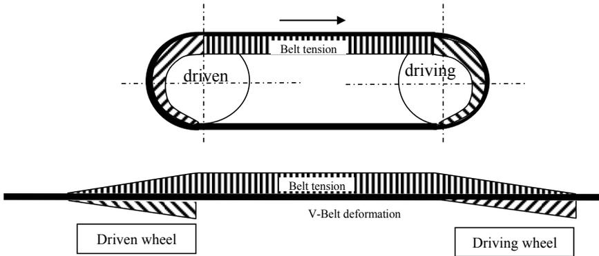
**Fig.10.** The tension and deformation of the belt on the wheel
