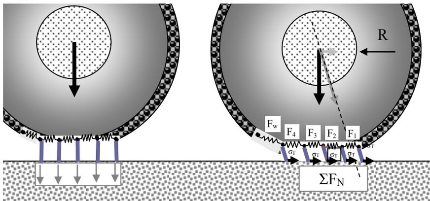
**Fig.5.** Force acting on no rotating wheel
