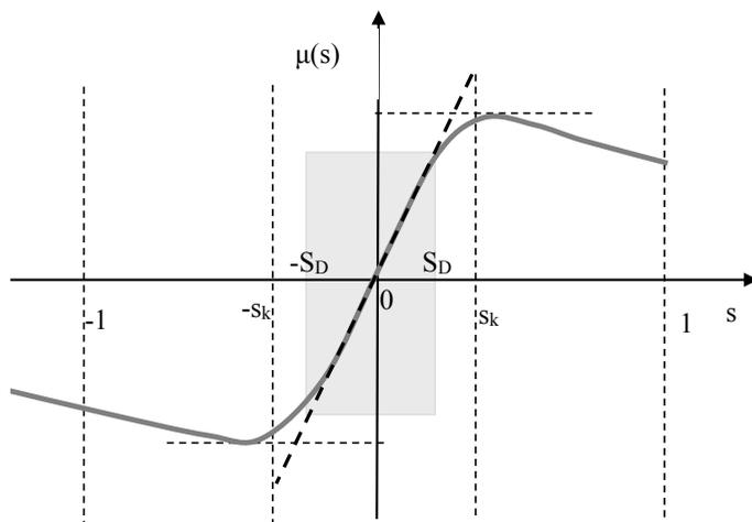
**Fig.2.** Classical relation curves of driving force coefficient ( $\mu$ ) to slip ( $s$ )  $\mu=f(s)$  with linear part of relation
