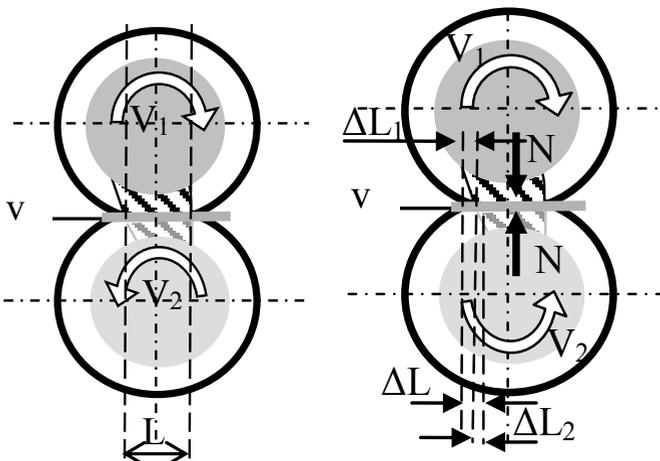
**Fig.11.** The wheel gear deformation
