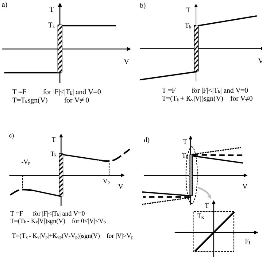
**Fig.8.** The Columbus friction model a) constant friction value during movement b) friction force increases with the speed c) the Stribeck effect –friction force decreases with the speed growing (the part for low sliding speed), d) the friction value as the answer for driving force in static state [12].
