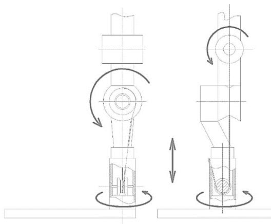
**Fig. 5** The mechanical ankle joint (patent pending)
