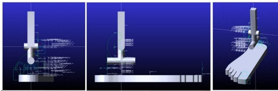
**Fig. 3** Simulation model of the knee joint in MSC Adams software
