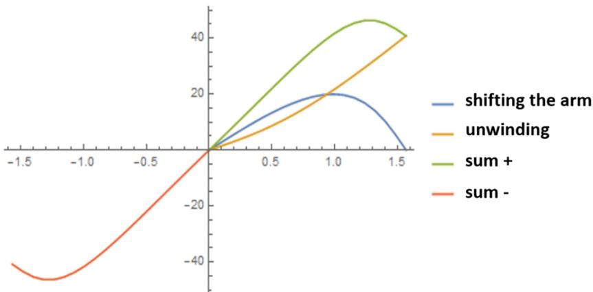
**Fig. 7.** Tension member length change due to ellipse rotation.
