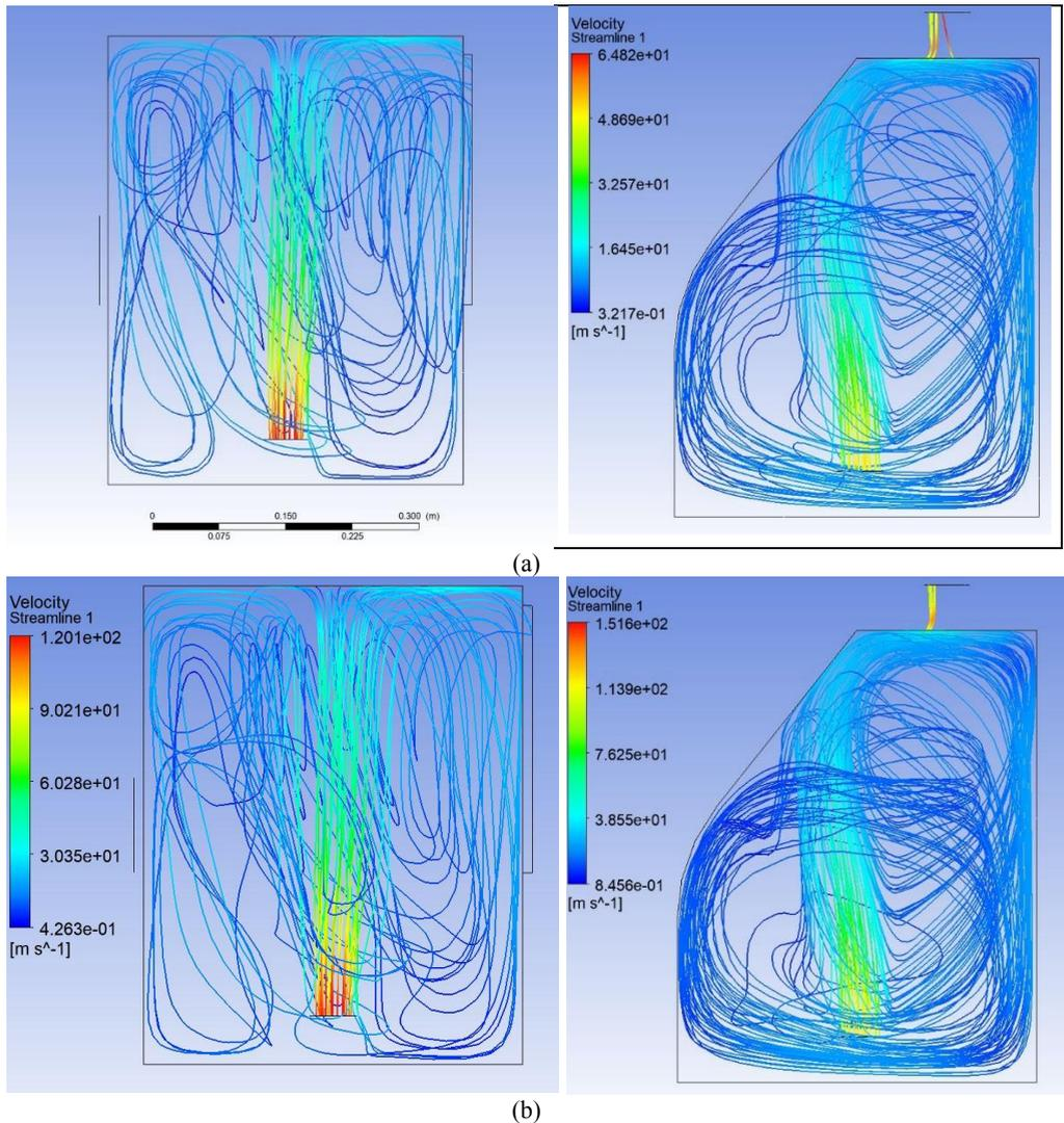
**Fig. 7.** (a) Left, Existing design mild cough velocity. Right, Improved design mild cough velocity, (b) Left, Existing design, strong cough velocity. Right, Improved design, strong cough velocity.
