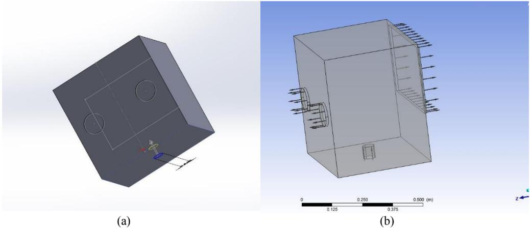
**Fig. 5.** (a) Location of nozzle inlet on bottom of box, (b) Inlet and Outlet Boundary Locations
