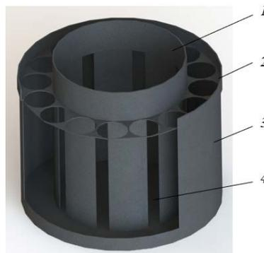
**Fig. 1.** A three-dimensional model of centrifugal separation device with coaxially arranged pipes (cross-section view): 1 – inlet nozzle of inner cylindrical pipe, 2 – grid with round holes, 3 – body of separation device, 4 – rectangular holes.
