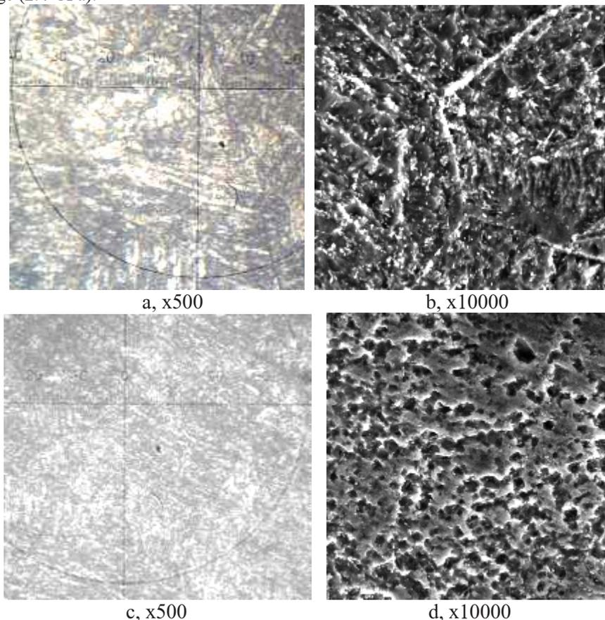
**Fig. 3** - Microstructure of the steel 15Cr12WNiMoV after the heat treatment in mode 2 (a, b) and in mode 3 (c, d)
