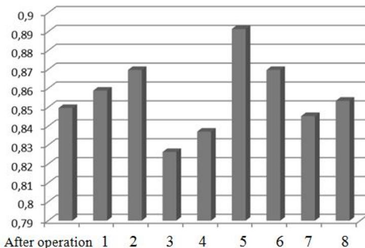
**Fig. 6.** Plasticity coefficient of the steel 15Cr12WNiMoV after the operation and the following heat treatment
