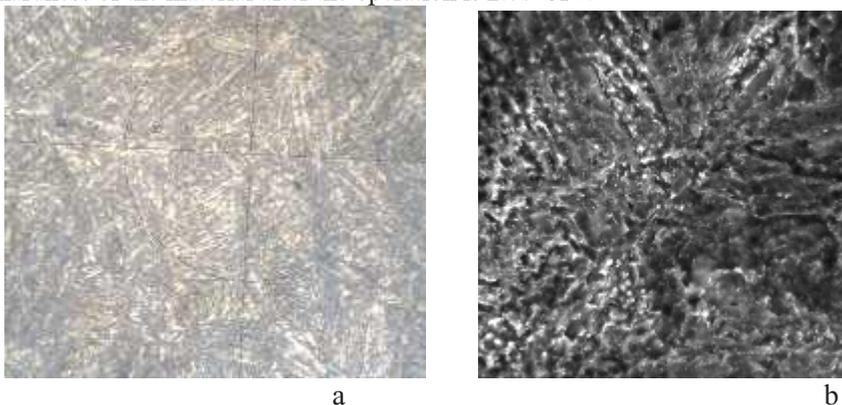
**Fig. 1** - Microstructure of the steel 15Cr12WNiMoV after the operation: a - x500, b- x10000
