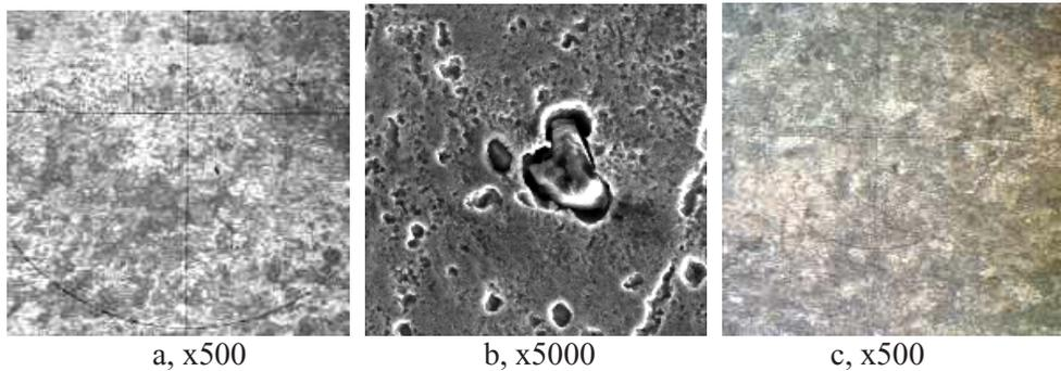
**Fig. 2** - Microstructure of the steel 15Cr12WNiMoV after the heat treatment in mode 1 (a, b) and mode 5 (c)
