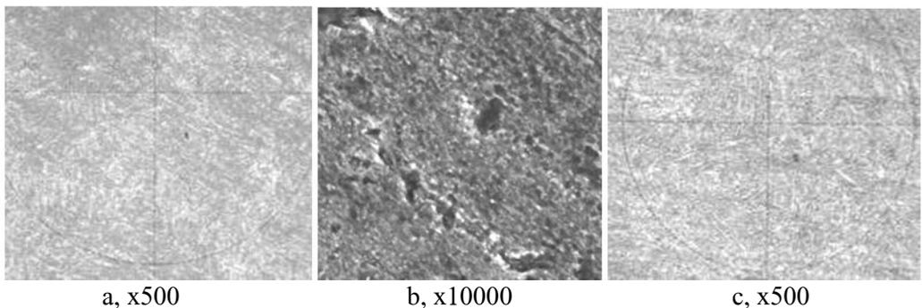
**Fig. 5.** The microstructure of the steel 15Cr12WNiMoV after the heat treatment in mode 4 (a, b) and in mode 8 (c)
