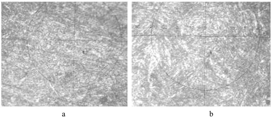
**Fig. 4.** The microstructure of the steel after the heat treatment: in mode 3 (a) and in mode 7 (b), x500
