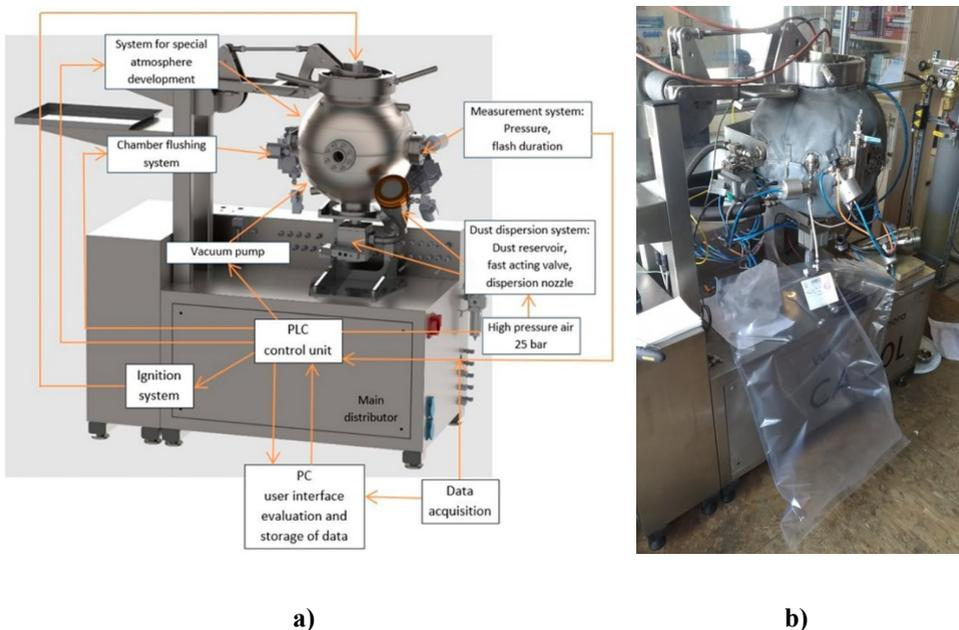
**Fig. 1.** Experimental setup a) the 20-L spherical vessel, b) gas sampling from Tedlar bag.
