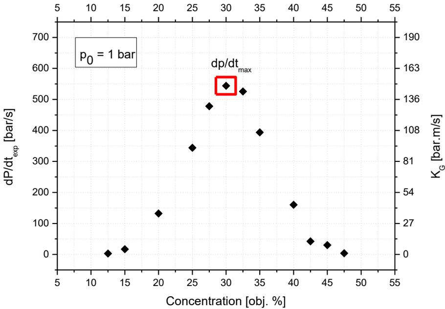
**Fig. 3.** Explosion pressure rise versus concentration.
