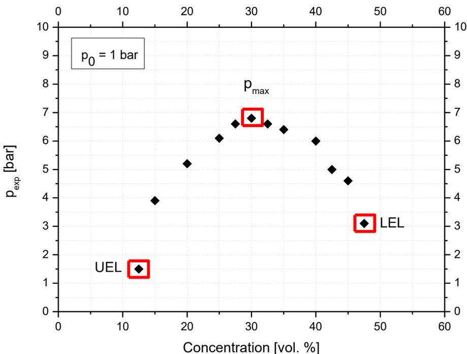
**Fig. 2.** Explosion pressure versus concentration.
