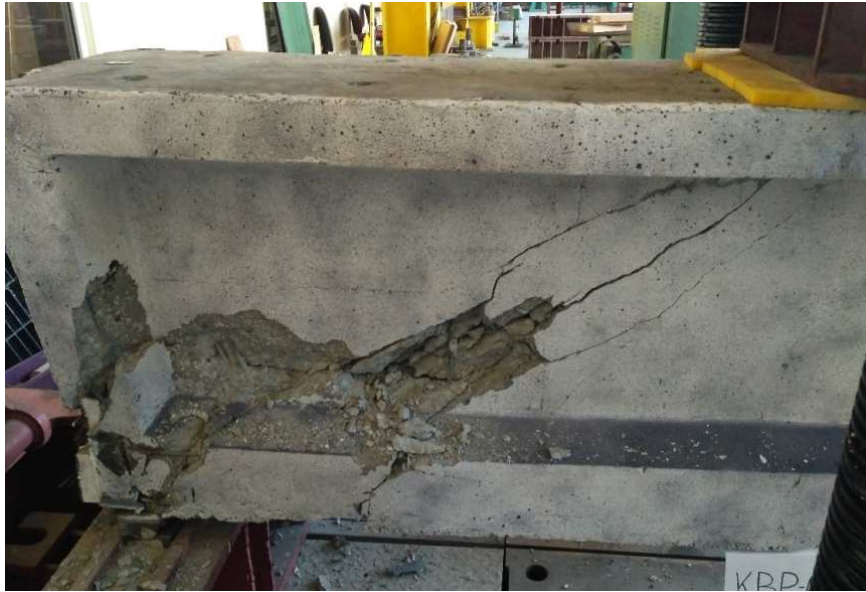
Fig. 5. Failure mode of KBP-01 specimen.
