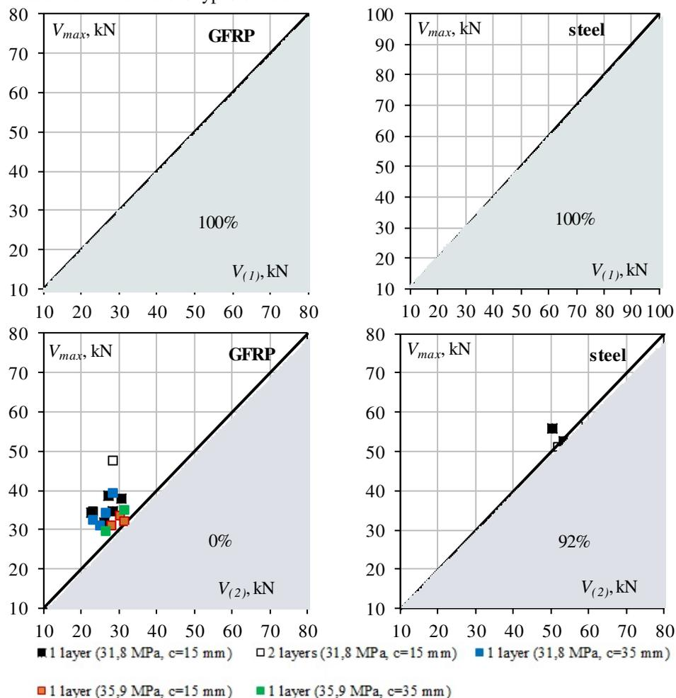
**Fig. 5.** The experimental and calculated shear capacity according to presented models
