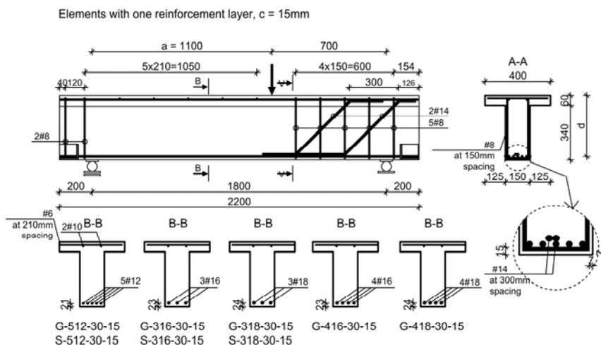
**Fig. 1.** Reinforcement of tested beams (series I, one reinforcement layer,  $c = 15$  mm)
