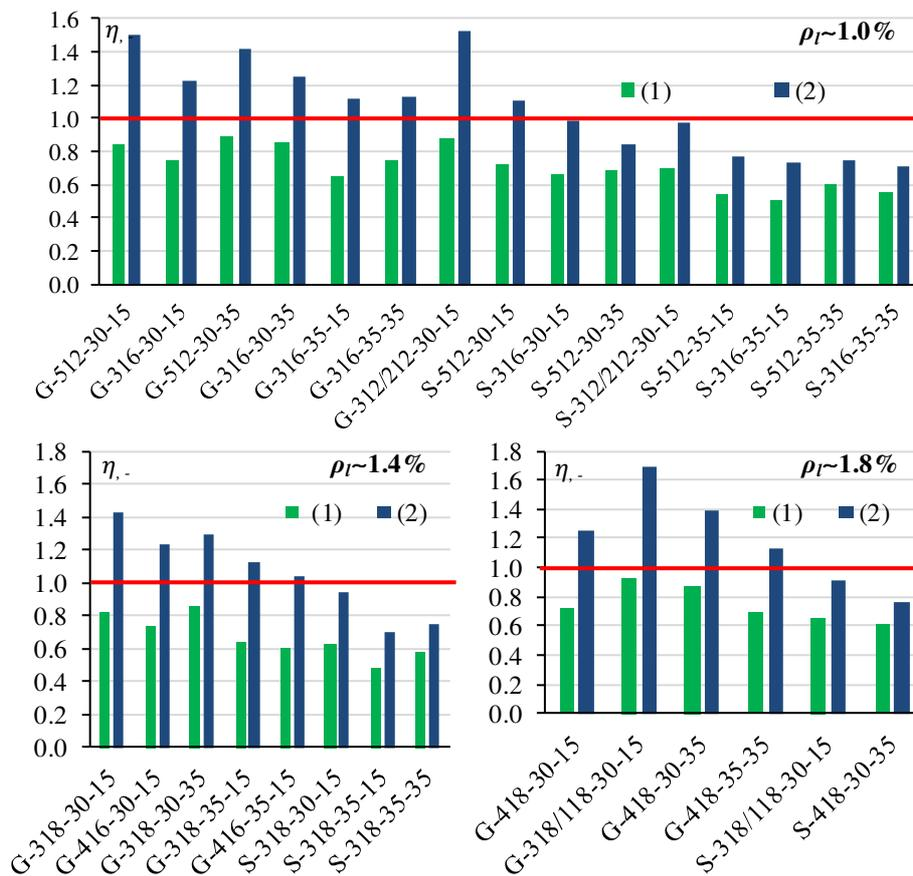
**Fig. 6.** The comparison of results for models [1] and [2] for longitudinal reinforcement ratio about 1.0, 1.4% and 1.8%
