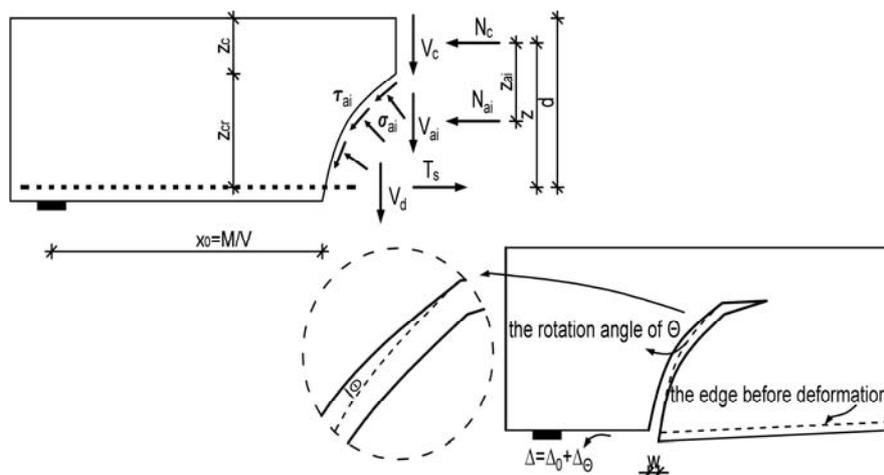
**Fig. 4.** The forces acting on the fragment of the beam and kinematic condition for critical crack
