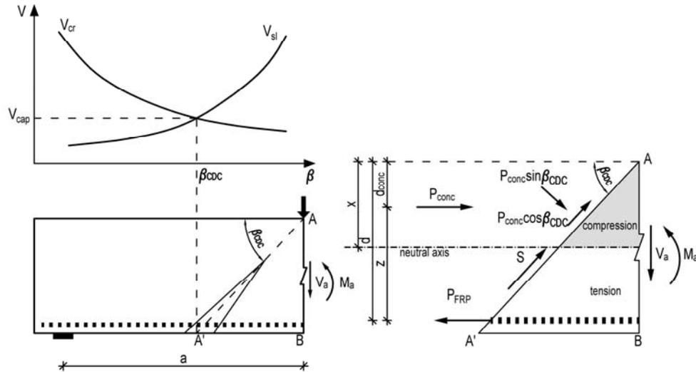
**Fig. 3.** The typical shear crack and forces acting on the fragment of beam in model [1]
