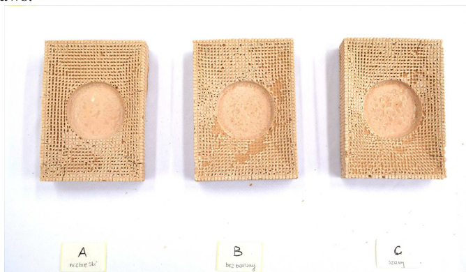
Fig. 4. Geopolymer castings with visible surface defects.
