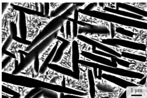
**Figure 3: SEM micrograph of the “Standard” microstructure after long-term ageing of 6000 h at 450 °C**
