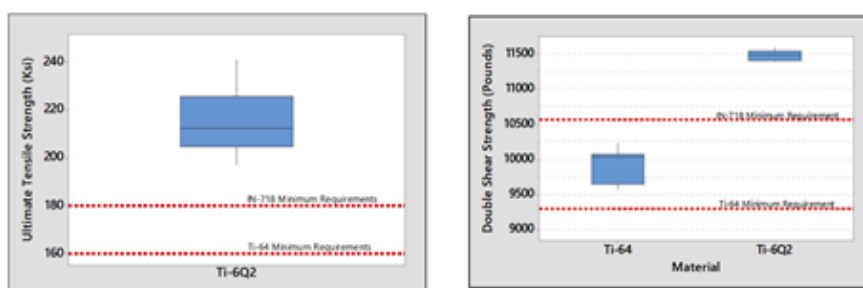
Figure 7: Tensile and double shear strength of Ti 6-22-22 (Ti-6Q2) fasteners compared with Ti 6-4 and IN-718.
