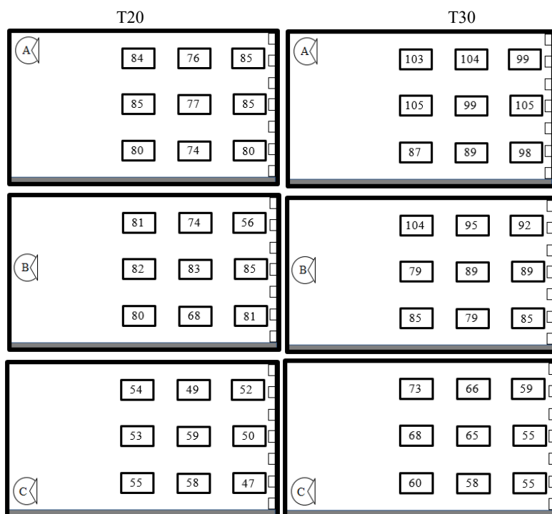
Fig. 3. Measured values of reverberation time T20 and T30 (ms) for different positions of the source and receiver in a room with a scattering test wall.
