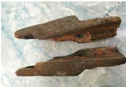
**Fig. 1.** Wear on chain surface.
