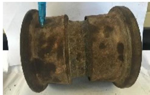
**Fig. 3.** Wear on surface of roller.
