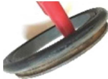
**Fig. 2.** Damage on oil seal for roller.
