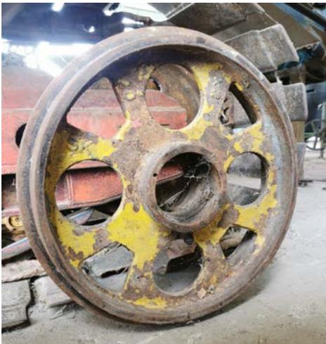
**Fig. 5.** Damage on wheel guide.
