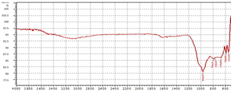
Fig. 7. Spectrogram of the corrosion deposition of the composition of sodium cyclotriphosphate with lanthanum in a ratio of 3:1.
