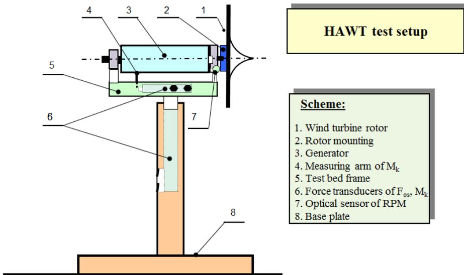
**Fig. 1.** Scheme of the HAWT test setup.
