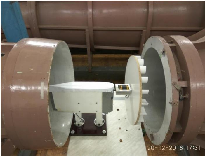
**Fig. 5.** Measurement setup during HAWT performance verification in the measurement section of the wind tunnel.
