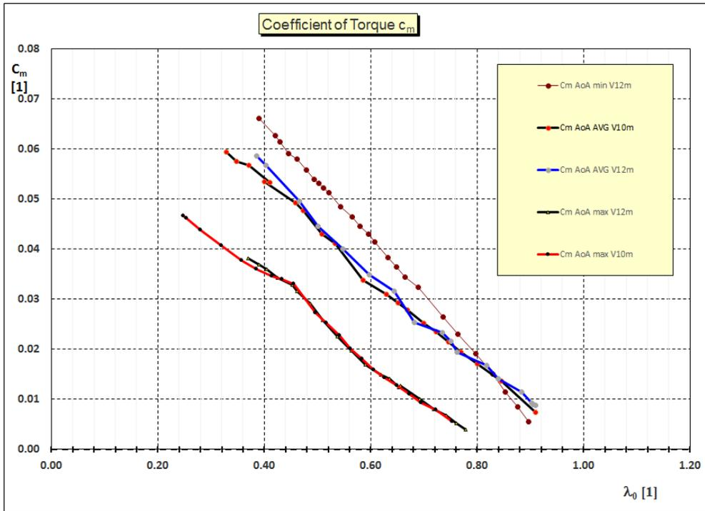
**Fig. 7.** Torque characteristics and impact of modifiable angle of attack of all blades.
