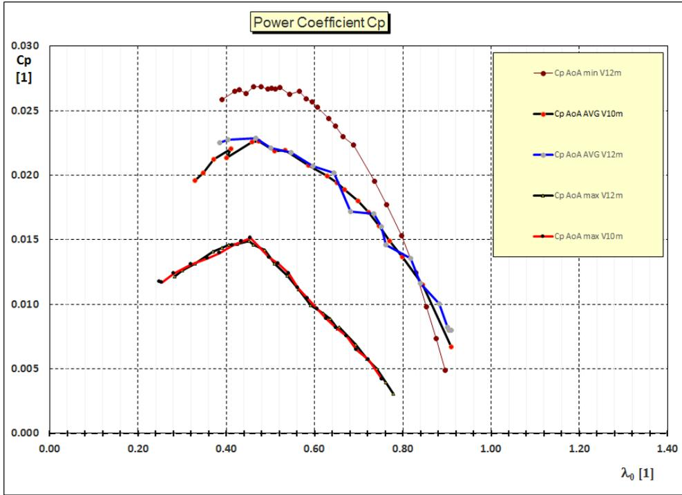
**Fig. 6.** Power coefficient dependency on tip-speed ratio  $\lambda_0$  and impact of the change of the angle of attack on the results.
