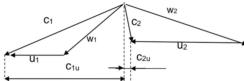
**Fig. 4.** Speed triangles on the wheel of the HAWT.
