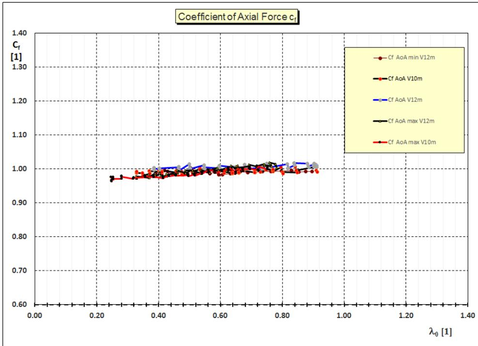
**Fig. 8.** Coefficient of axial force plotted against tip-speed ratio  $\lambda_0$ . The impact of variable angle of attack of all blades can be clearly seen from both graphs.
