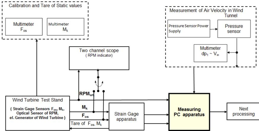
**Fig. 2.** Scheme of the measurement chain.
