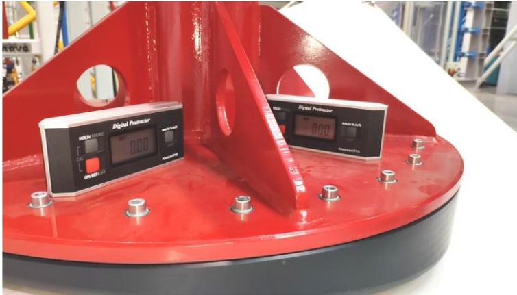
**Fig. 3.** Levelling the load piston.
