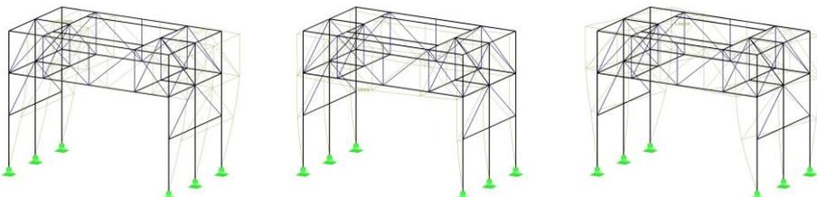
**Fig. 9.** Model 3 – first three eigenshapes.
