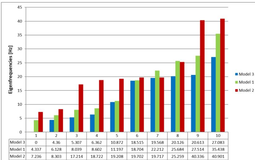
**Fig. 5.** Eigenfrequencies of Models 1, 2, 3.
