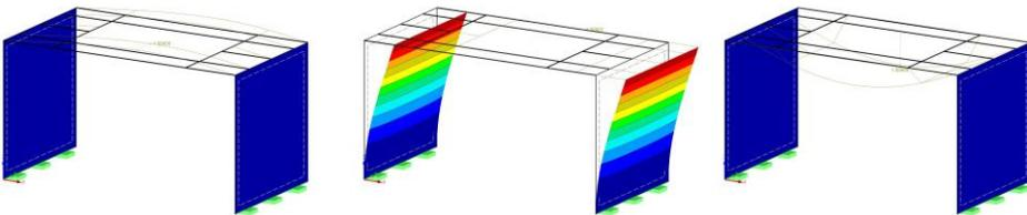
**Fig. 8.** Model 2 – first three eigenshapes.
