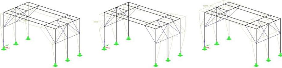
**Fig. 7.** Model 1 – first three eigenshapes.
