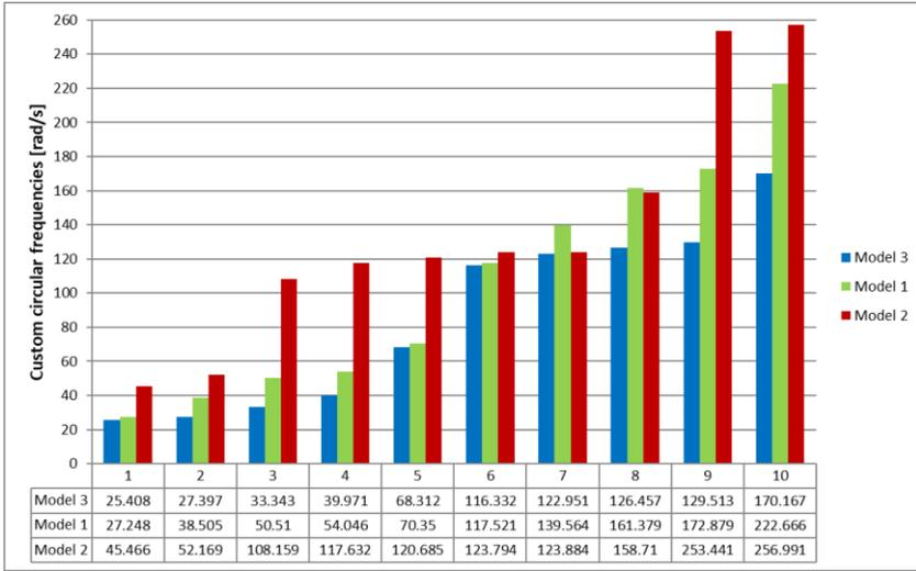
**Fig. 6.** Circular eigenfrequencies of Models 1, 2, 3.
