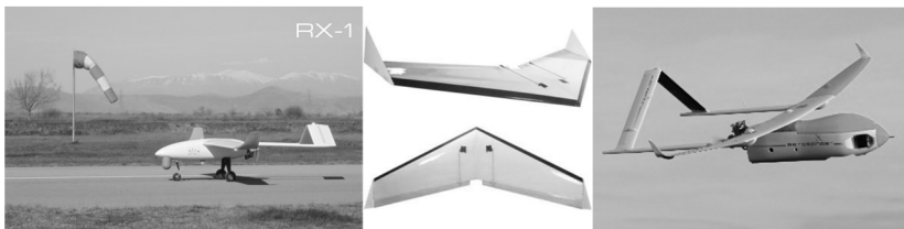
Fig. 3 (left) The HCUAV. (middle) The Zagi Flying Wing UAV. (right) The Aerosonde UAV.
