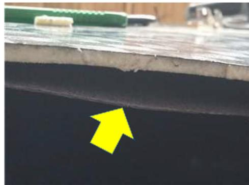
**Fig. 3.** Delamination of the integral tank cover
