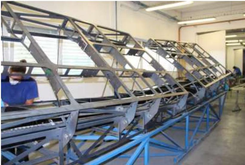
**Fig. 10.** Metal bonding jigs of the wing
