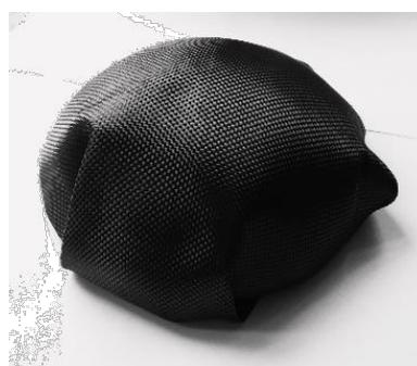
**Fig. 11.** Carbon Fiber Weave Fabric
