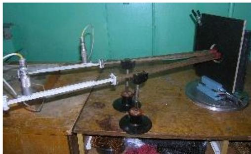
**Fig. 9.** Determination of the shielding properties of polymer composites.
