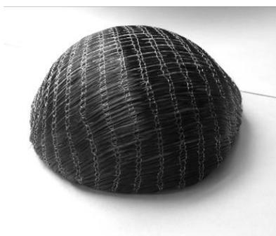
**Fig. 10.** Carbon weft-knitted fabric
