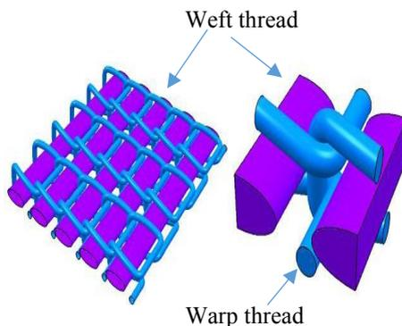
**Fig. 2.** Rib 1+1 with weft thread, produced on upgraded machine
