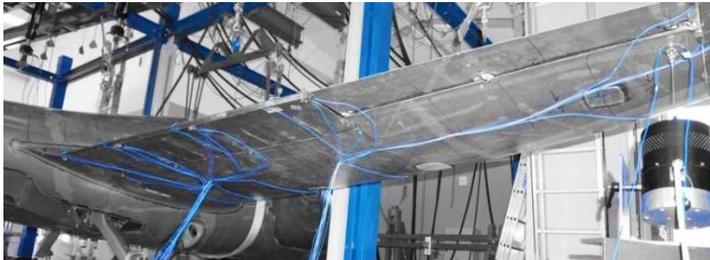
**Fig. 8.** View on bottom side of right wing during test on Flaris Lar-1.
