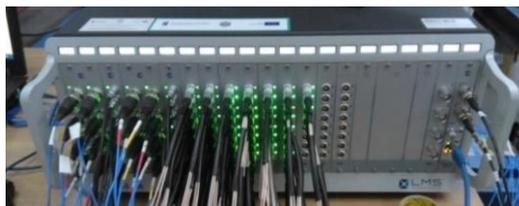
**Fig. 2.** Modal analyzer LMS SCADAS Lab with wires connecting piezoelectric sensors.
