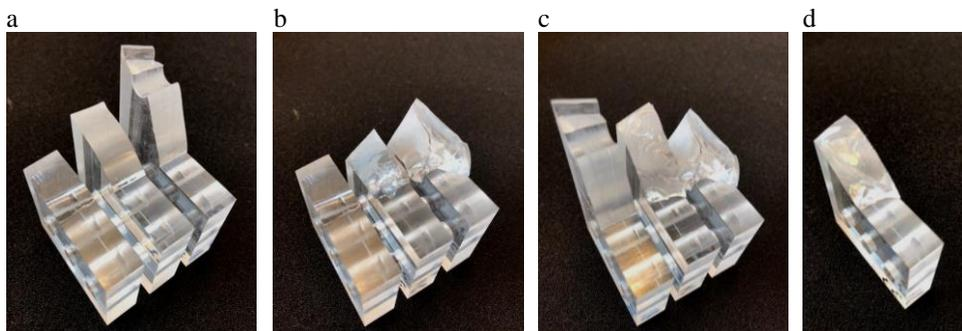
**Fig. 3.** Representative fractured CTS specimens under different loading conditions; from left to right (a) mode I, mixed mode I/II, mode II, (b) mode I, mixed mode I/III, mode III, (c) mode II, mixed mode II/III, mode III, and (d) mixed mode I/II/III.
