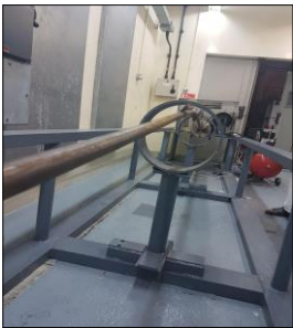
Fig. 8. Large lateral amplitude for 1" drillstring near its rotational critical speed.
