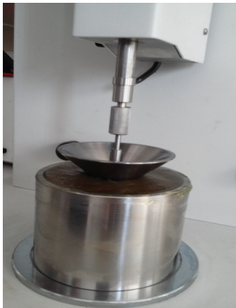
Fig. 9. Laser penetrometer PL-12DC – view during the test [7]
