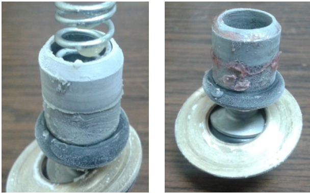
Fig. 11. View of the used Elf MULTI grease (on the left) and Vecolite EPX 00 grease (on the right) in the relay valve operating at temperature of -26^{\circ} [7]
