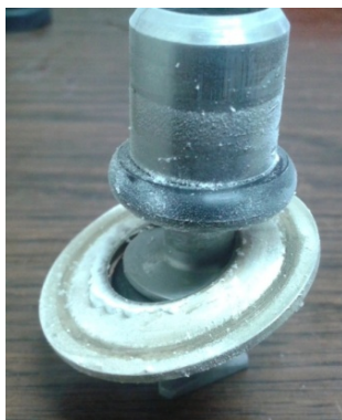
Fig. 13. View of the used TF silikon + teflon grease in the relay valve operating at temperature of -26^{\circ}\text{C} [7]
