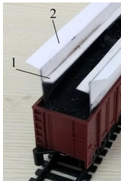
Fig. 4. Model of the open wagon with additional boards (model without front side additional board): 1 - “internal wing”; 2 - “external” board
