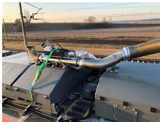
Fig. 3. Flowmeter mounted on the roof of the vehicle and the heated line for gas sampling
