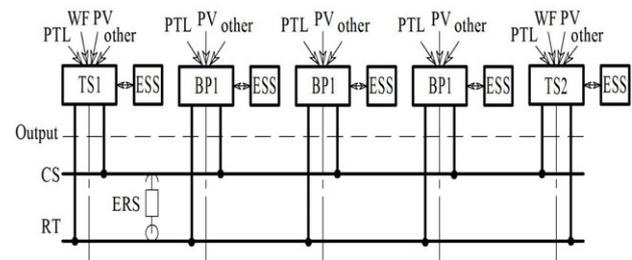
**Fig. 4.** Block diagram of an electric hub: TS – traction substation; BP – boost point; RT – rail track; CS – catenary system; ESS – energy storage system; PTL – power transmission line; WF – wind farm; PV – photovoltaic power station; ERS – electric rolling stock.
