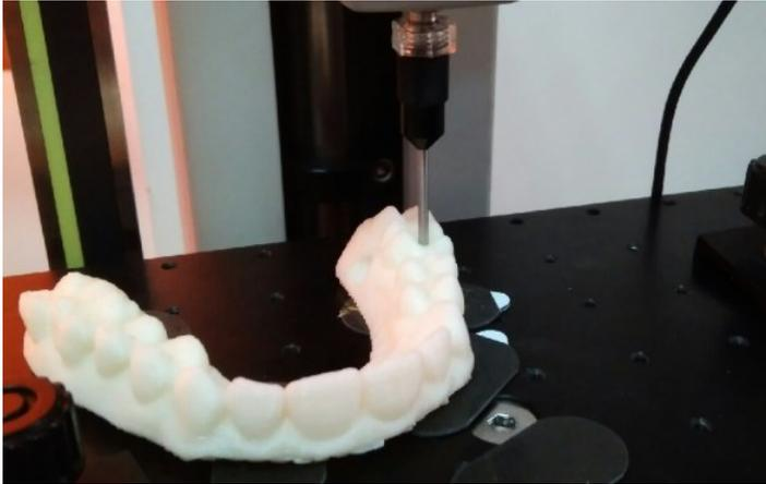
**Fig. 10.** ABS medical dental model acted with the penetrating pin gauge
