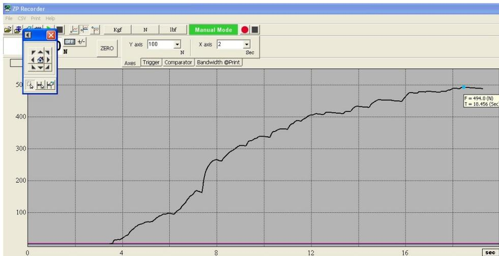
**Fig. 5.** Evolution of force in function of time of biocompatible thermoplastic dental prototype in the molar region
