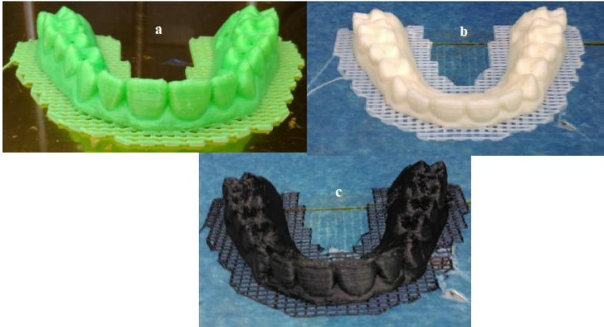
**Fig. 1.** Dental models realized by fused deposition modeling from different materials: a – ABS; b – ABS medical; c – PETG reinforced with carbon fiber [5, 7].
