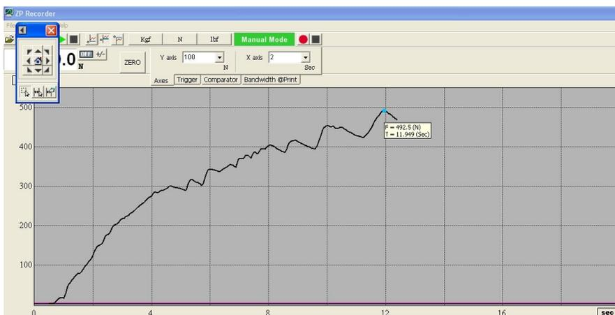
**Fig. 7.** Evolution of force in function of time of biocompatible thermoplastic dental prototype in the incisive region
