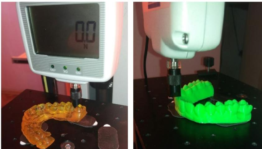
**Fig. 4.** Dental models on Test Stand HV-500N
