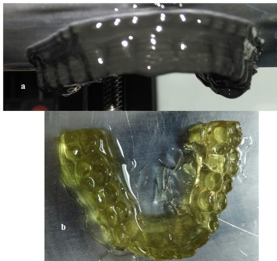
**Fig. 2.** Dental model realized by digital light processing technology from different materials: a – Wanhao Standard Resin; b – Industrial blend resin [7].
