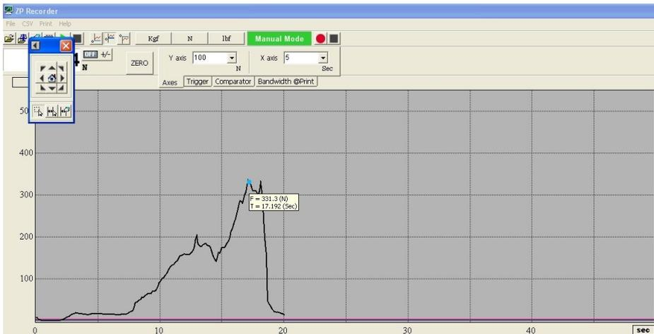
**Fig. 9.** Evolution of force in function of time of standard resin dental prototype in the incisive region
