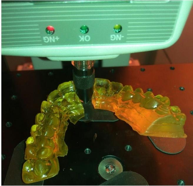
**Fig. 8.** The breaking of the photopolymer resin dental model.
