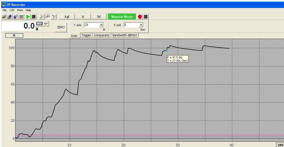
**Fig. 11.** Results of force in function of time of ABS (top) and ABS medical (bottom) prosthetic dental models tested with penetrating pin gauge
