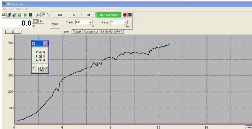
**Fig. 6.** Evolution of force in function of time of industrial resin dental prototype in the molar region.
