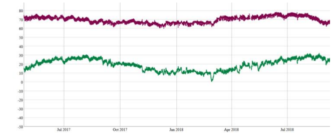
Fig. 21 Temperature ( ^{\circ}\text{C} , green curve) and relative humidity (%) in the beam (purple curve).
