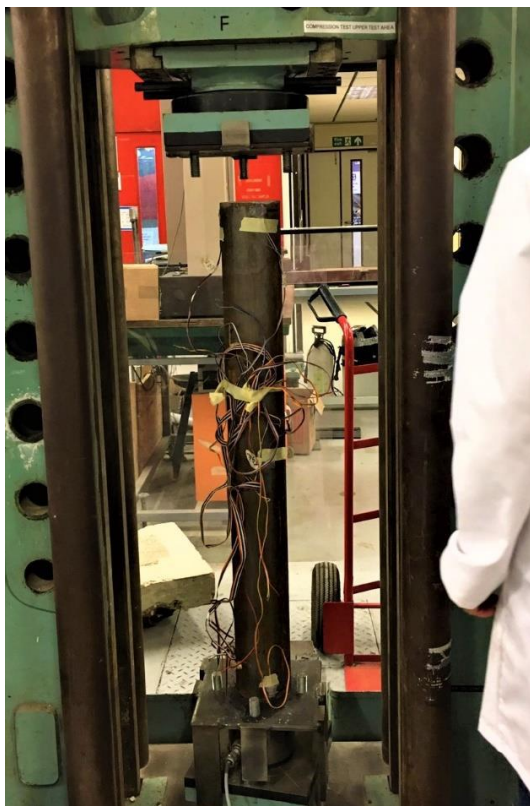
Fig. 3. Test setup for testing columns under compression.
