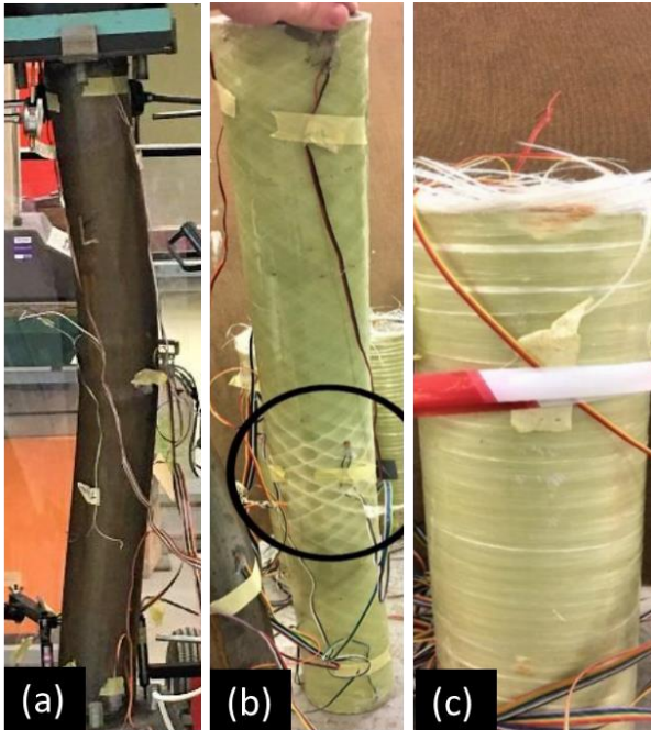
Fig. 5. Failure mode of all samples (a) steel (b) FRP-45 (c) FRP-90.
