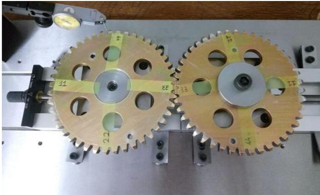
Fig. 15. Test spur gear pair & 4 main cases.
