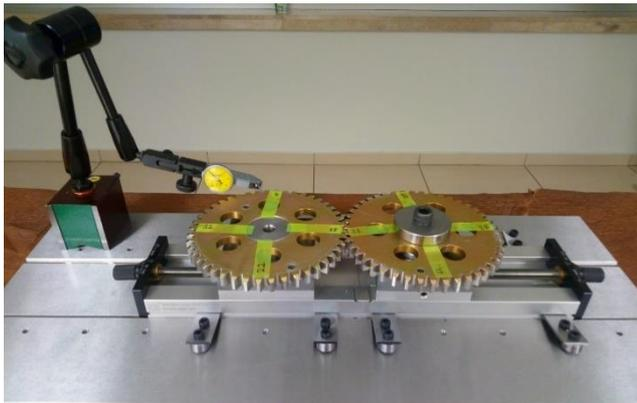
Fig. 14. Test rig & dial indicator.
