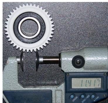
Fig. 3. Span measurement using a disc micrometer [3].
