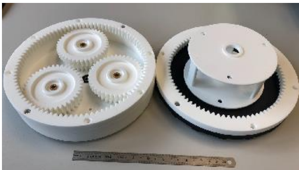
Fig. 6. Set of Wolfrom gearwheels and carrier cage in Alpha-I prototype.
