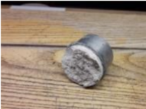
Fig. 8, 9. ‘Pull off’ samples for strength tests.
