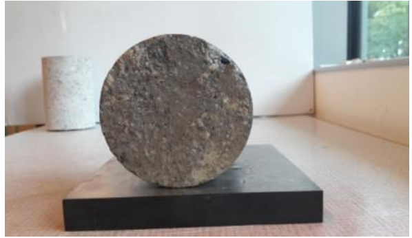
Fig. 7. Sample cut from the concrete slab, bonding layer.
