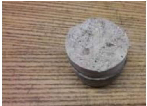
Fig. 7. Sample cut from the concrete slab, bonding layer.
