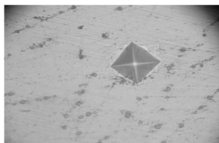
**Figure 3.** The hardness test of the surfacing layer.
