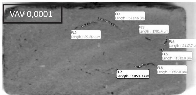
**Figure 7.** Sample crack measurements.
