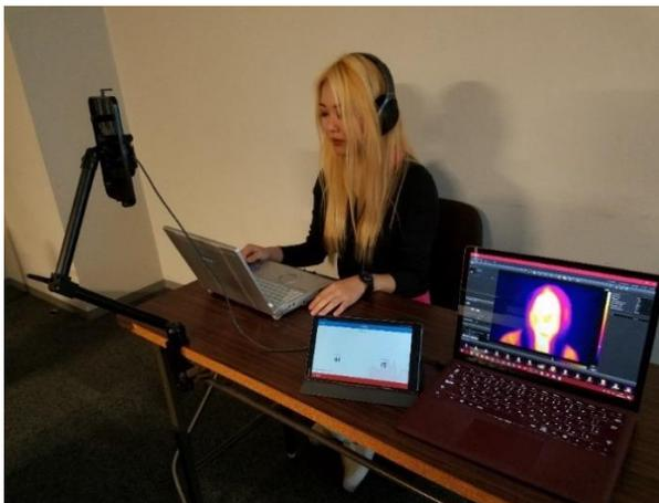
**Fig. 3.** Evaluation experiment recording a thermal video of face over watching a video clip
