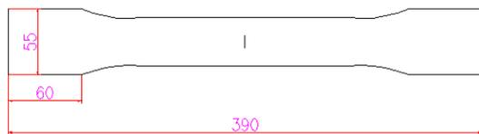
Fig.8 Specimen size
